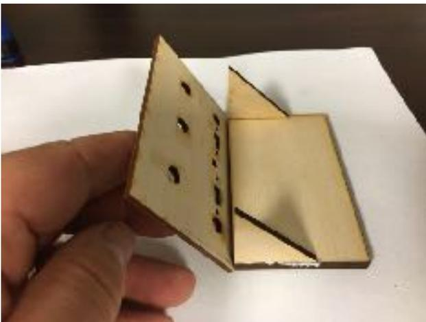
The front panel needs to overlap the base and triangular supports by 1/8th inch on each side.
