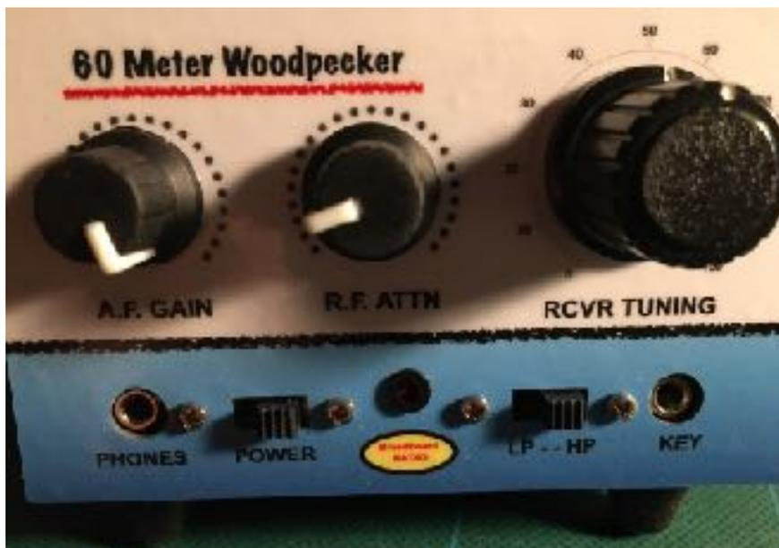
Push the LED mounting clip through the LED hole from the front of the panel. Use the screwdriver from behind to push the LED into the clip, but not all the way! The LED lens must be recessed part way.
