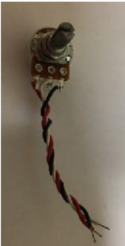
Prepare the Tuning pot with three 2 inch (red, white and black) wires as shown. Strip 3/8 inch of insulation from each end. Make good mechanical connections before soldering. Then twist the wires together as shown.
