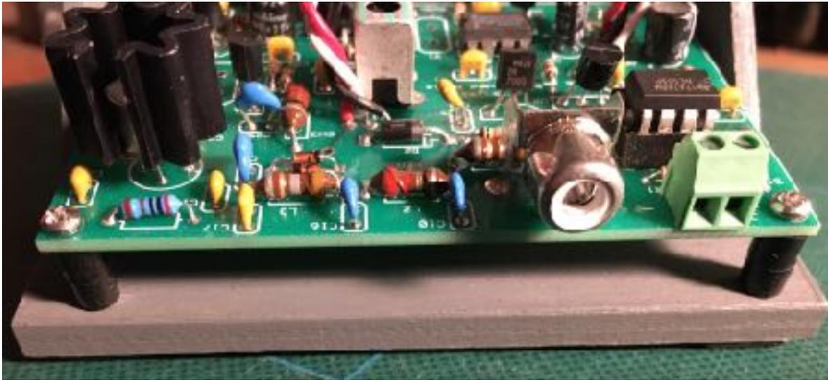
From the top of the circuit board, drill a 1/16 inch mounting hole using the corner mounting holes in the circuit board as a guide. It will not matter if the drill bit goes all the way through the wood.
