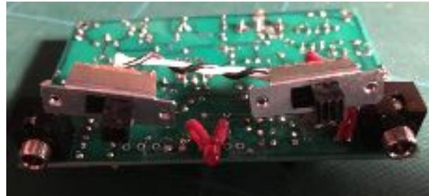
**Note: Place a piece of electrical tape over the circuitboard side of the switches to prevent shorts with the circuitboard traces!**
