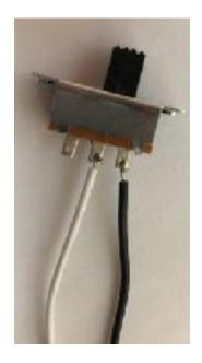
Prepare SW2 with 2 inch black and white wires. Strip 3/8 inch of insulation from each end. Make good mechanical connections before soldering. Then twist the wires together. Solder the other ends of the wires to the two holes labeled SW2. Note that the wires go through the Bottom of the circuit board and are soldered from the top. The wires may go in either of the two holes.
