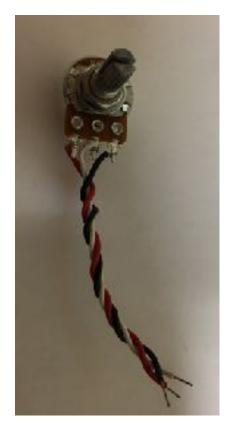
Prepare the Tuning pot with three 2 inch (red, white and black) wires as shown. Strip 3/8 inch of insulation from each end. Make good mechanical connections before soldering. Then twist the wires together as shown.
