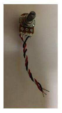
Prepare R.F. Attenuation pot with three 2.5 inch (red, white and black) wires as shown. Strip 3/8 inch of insulation from each end. Make good mechanical connections before soldering. Then twist the wires together as shown.
