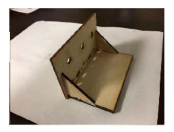
Once the glue has set, let the finished base and front panel cure for at least 15 minutes. The edges where paper is attached should be lightly sanded to remove the paper and prepare for painting. I like to use satin grey with a brush, but you may use any color you prefer brush or spray. If you paint the edges of the wood parts, I suggest sanding first to remove some of the dark color left by the laser cut.
