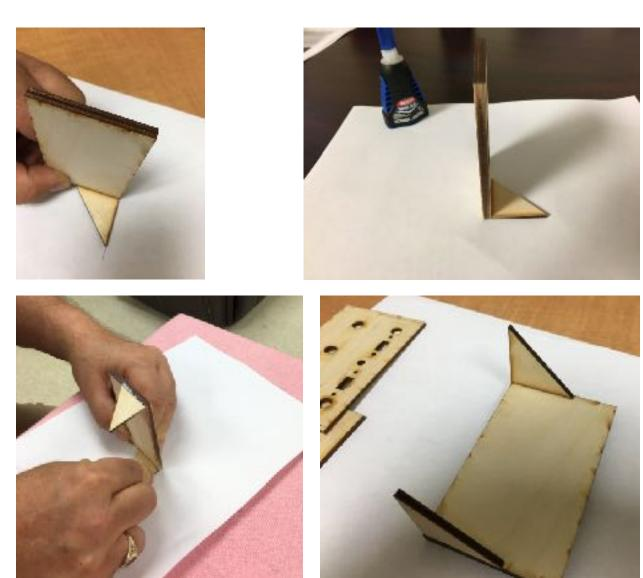
STEP 2. The base, now with the two triangular side supports, will be glued to the front panel. It needs to be centered so that the triangular supports and base leave 1/8th inch of space on each side.
