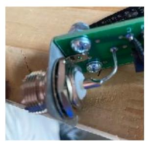
Attach the center insulator using two long machine screws, two lock washers, two ring terminals, two nuts and two lock nuts as shown. The machine screws will self tap through the circuit board.
