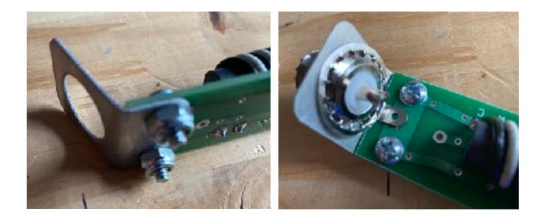
Tighten the nut onto the coax connector. A large box wrench will work well. Then bend the bracket to 90 degrees.
