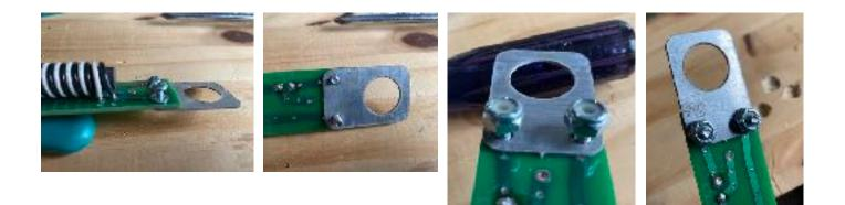
Bend the Aluminum bracket upward about 45 degrees. Place the coax connector through the hole and secure with the lock washer and mounting nut. The solder tab on the locker will need to be bent with pliers about 90 degrees so that the mounting bracket can be bent to 90 degrees after the coat connector is tightened.
