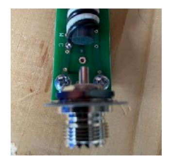
Once the bracket is in place, strip a remaining piece of wire and fashion as shown to connect the center of the coax connecter to the circuit board and secure with solder. Trim the excess wire from the bottom of the circuit board.
