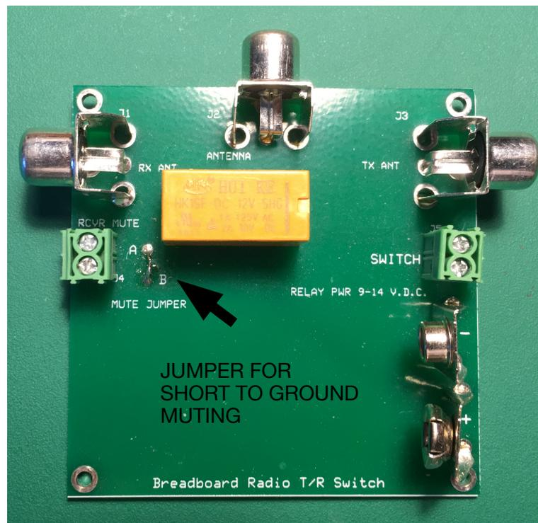
will use “open circuit” muting on transmit. If you require “short to ground” on transmit for receiver mute, you will need to solder a wire jumper between points “A” and “B” on the circuit board. Use the wire supplied and strip each end before soldering.
