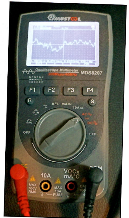
Mustool MDS8207 scope / meter displaying an audio waveform.
