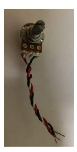
Prepare the Tuning pot with three 2 inch (red, white and black) wires as shown. Strip 3/8 inch of insulation from each end. Make good mechanical connections before soldering. Then twist the wires together as shown.
