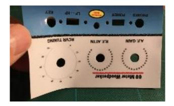
Note that the decal has overlap on all four sides. Lay the front panel face down on a clean firm surface like a cutting board or firm piece of cardboard. Use the hobby knife to trim off the overlapping sides of the decal. Use the edges of the front panel wood as a guide.
