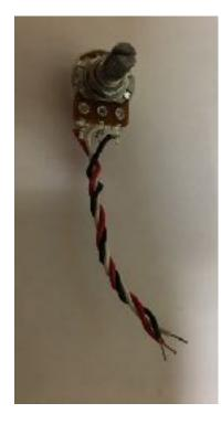
Prepare R.F. Attenuation pot with three 4 inch (red, white and black) wires as shown. Strip 3/8 inch of insulation from each end. Make good mechanical connections before soldering. Then twist the wires together as shown.
