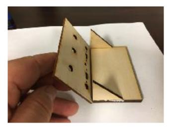
The front panel needs to overlap the base and triangular supports by 1/8th inch on each side. This will allow the side panels to fit properly.
