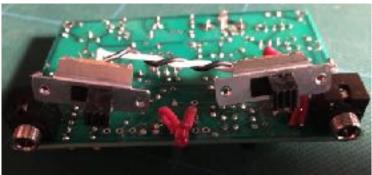
Note: Place a piece of electrical tape over the circuitboard side of the switches to prevent shorts with the circuitboard traces!
