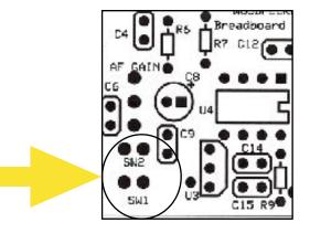
Prepare SW2 with 4 inch black and white wires as in SW1 (above). Solder the other ends of the wires to the two holes labeled SW2. Note that the wires go through the Bottom of the circuit board and are soldered from the top. The wires may go in either of the two holes.
