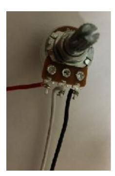
Prepare A.F. Gain pot with three 2 inch (red, white and black) wires as shown. Strip 3/8 inch of insulation from each end. Make good mechanical connections before soldering. Then twist the wires together as shown in next step photo.
