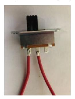
Prepare SW1 with two 2 inch red wires as shown. Strip 3/8 inch of insulation from each end. Make good mechanical connections before soldering. Then twist the wires together as shown. Solder the other ends of the red wires to the two holes labeled SW1. Note that the wires go through the Bottom of the circuit board and are soldered from the top. The wires may go in either hole.
