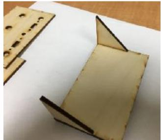
STEP 2. The base, now with the two triangular side supports, will be glued to the front panel. It needs to be centered so that the triangular supports and base leave 1/8th inch of space for the side panels to be mounted.
