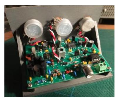
Position the circuitboard on the bottom of the cabinet as shown. Slide forward while aligning the phone and key jacks, switches and LED to fit through the front panel holes. Using a small flat blade screwdriver below the circuit board may aid in aligning the switches and LED to fit in the holes.
