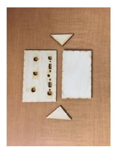
STEP 1. Attach the two triangular supports to the base (1/4 inch thick rectangle). Use a sheet of copier paper to work on. Lightly sand the edge to be attached. Apply glue to the edge to be glued. Align the the two surfaces as shown and firmly hold in place for two or three minutes. The pieces must join as close to 90 degrees as is possible. Once the glue is set, leave it still to cure for five minutes.
