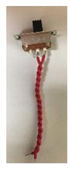
SW2 high-low pass audio switch (SPDT)
