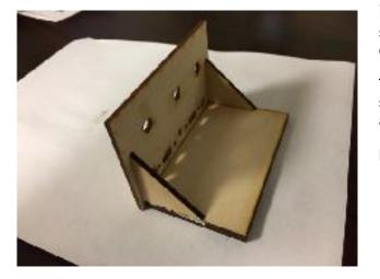
Apply glue to the front edges of the base and triangular supports. With the base sitting flat, align the "centered" front panel and hold in place for about two minutes.
